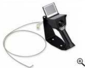
Pegasus 3.9mm Aviation Ready articulating Video Borescope
